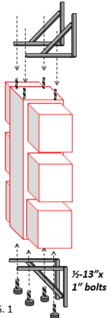
Figure 1 shows a wall mount, it can be mounted with a simple angle frame on the bottom or the top or both.
